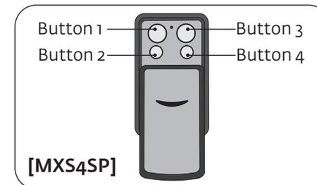
**NOTE:** If you select a button other than the n° 2 for pedestrian opening, the control board will recognize it as complete opening button, which means it will override the first pressed button. If the pedestrian opening is not wished, do not press the n°2 button and wait for the CODE LED to turn off.
