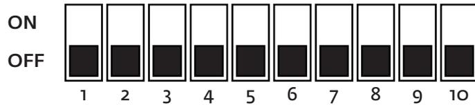
NOTE: The control board in standard mode has all the dippers in OFF mode.
